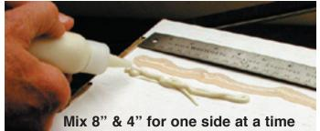
4) Mix Hotcha 2:1 ratio; An 8" bead of the amber glue mixed with a 4" bead of the white catalyst will do each side.
