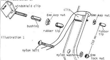
Note For reasons of structural strength, the windshield must be "preloaded" (slightly bent) before the top holes in the fairing will line up with the clip stud.
