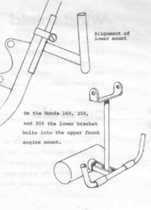
Install the fairing. With the machine on its center stand, lift the front wheel and slide the fairing under the tire.
