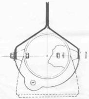
Install the headlight; tighten all bolts.
